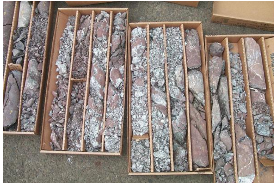
Core from a fault zone in the Triassic Stockton Fm, (USGS)
